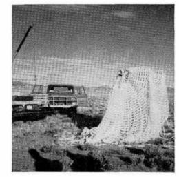
RIBBON CHUTE used in recent test is shown draped over instrumentation payload after impact at Tonopah Test Range.
